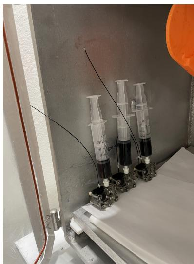
Let them sit in this vacuum for about 30 seconds. Remove the molds and inject more rubber. Repeat this process of vacuum and injection at least 3 times.
