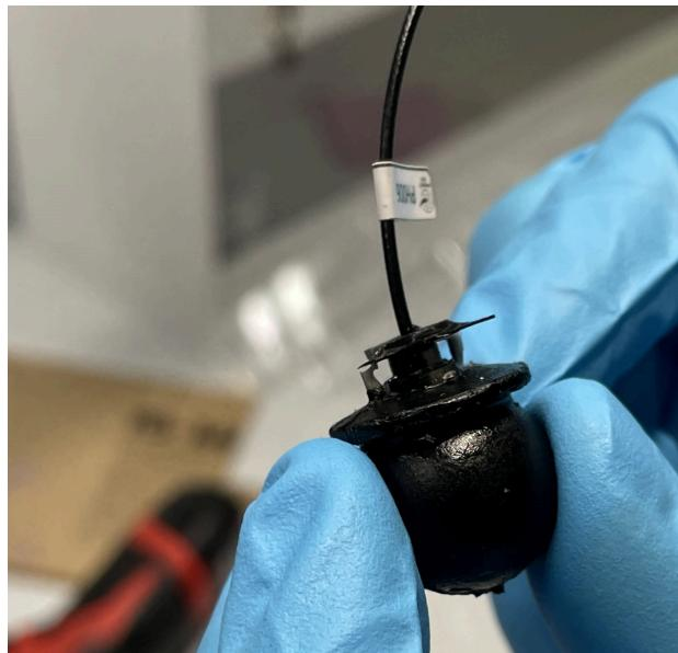
Notice that some rubber has cured where the air holes were and around the wire. The standoff flange is also still attached.
