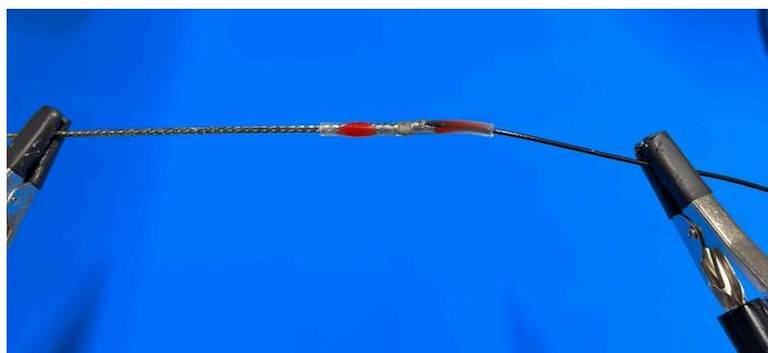
3. The next step is to create the supporting wire. Cut 50 mm from the steel cable and cover it in about 55 mm of the 0.13" moisture resistant heat shrink. Inject sil poxy into each end of the heat shrink and then use the heat gun to shrink the heat shrink around the steel cable.
